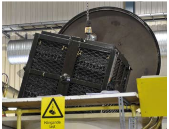
Process basket ready for cold wash station after impregnation in autoclave
