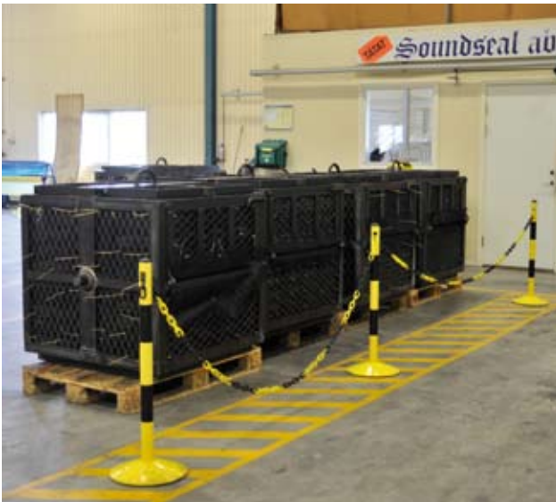
Impregnated castings in process baskets ready for visual inspections prior to returning to the customer
