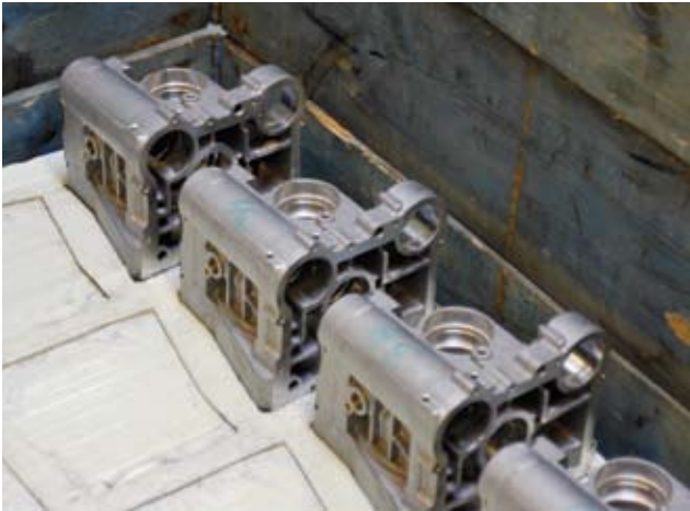
Packing of impregnated castings
