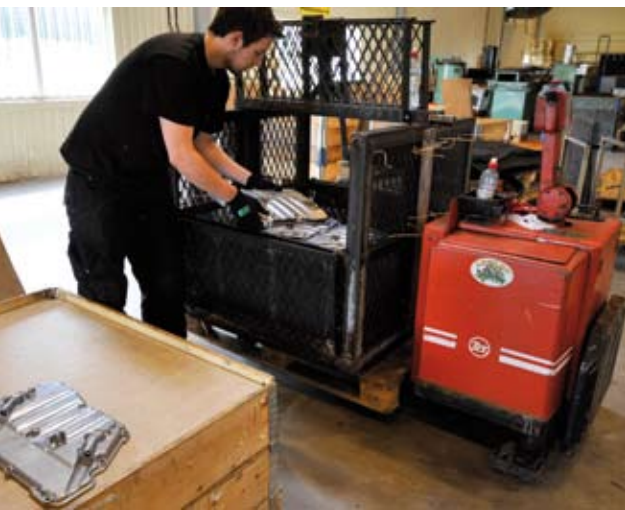
Visual inspection of castings
